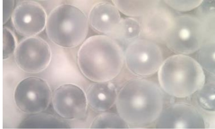
Figure 1. Improved 100% dense ADN prills with reduced sensitivity.
