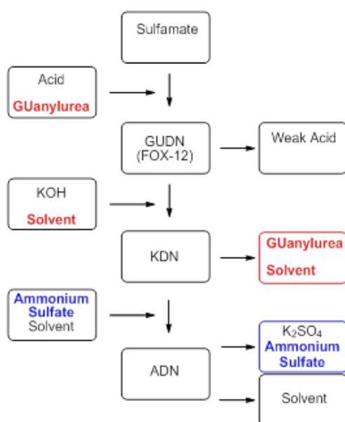
Figure 2. ADN production process at EuB
