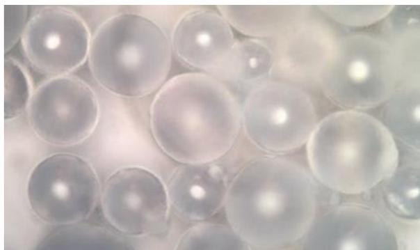
Figure 3. Improved 100% dense ADN prills with reduced sensitivity.
